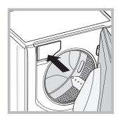
The detergent dispenser drawer is located inside the machine and can be accessed by opening the door.
